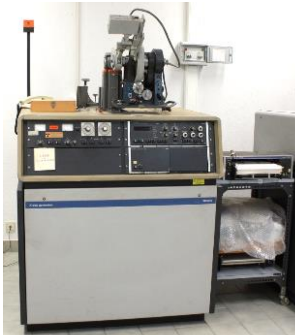
Philips PW 1500 powder diffractometer (Bragg-Brentano geometry), equipped with a large-anode copper tube operating at 50 kV - 40 mA and a curved graphite crystal monochromator
