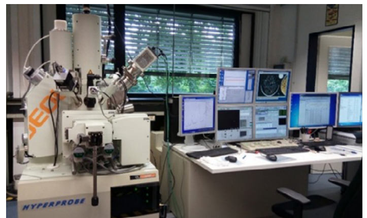
Figure 34: Left: BGR headquarters as one of three institutes in the GEOZENTRUM HANNOVER; Right: JEOL XA-8530F Hyperprobe for electron probe microanalysis.
