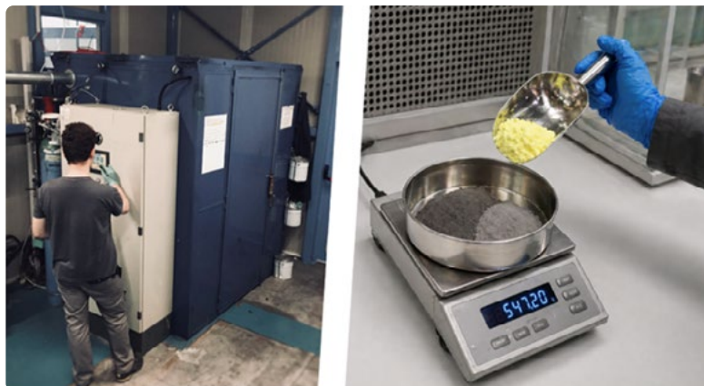
Figure 3 | Mechanochemical synthesis of tetrahedrite concentrates to produce powdered compositions suitable for consolidation of preforming TE material samples.
